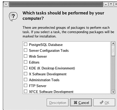
Figure 5-3 Marking package groups for installation
